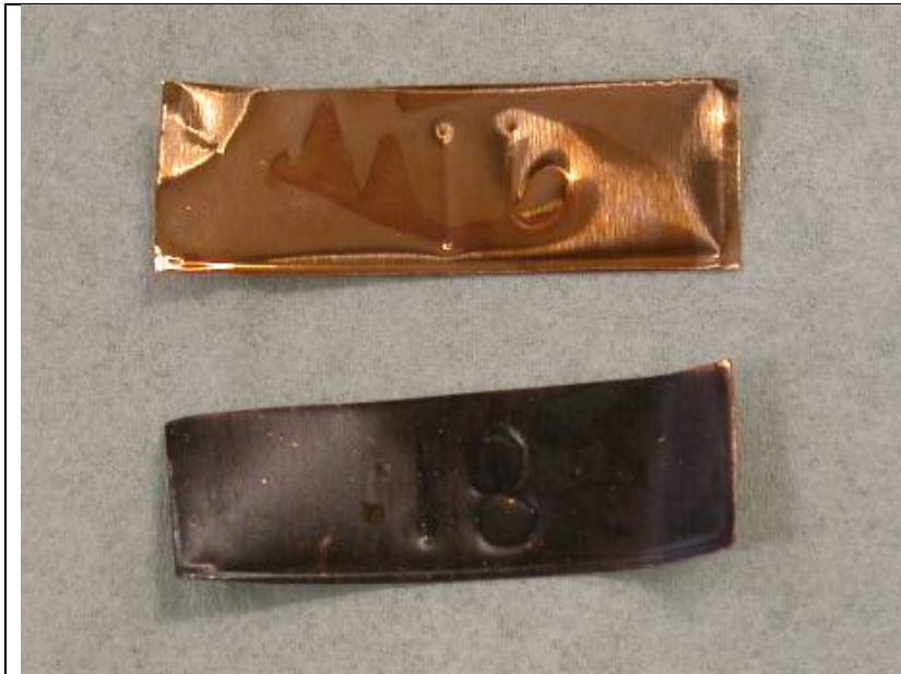
Figure 12. Copper strips used to measure corrosion during the phosphine combination treatment, top strip in mill in sealed electrical box, the bottom strip was in the fumigated area, Mill 6.
