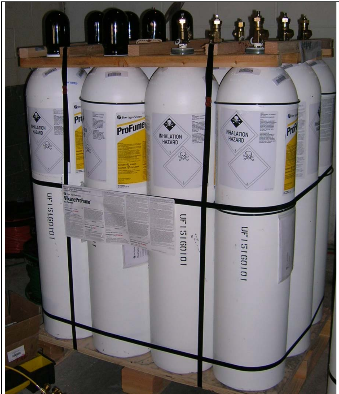
Figure 4. Cylinders of sulfuryl fluoride gas (ProFume) used in treatments in Mills 4, 5 and 8.
