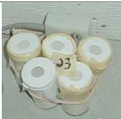
Figure 10. Vials with red flour beetle ( Tribolium castanenum ) adults and eggs used for bioassays and a temperature data logger.
