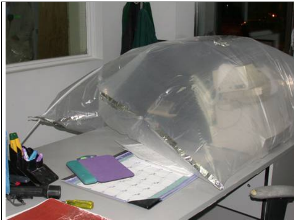
Figure 6. Computer equipment sealed and pressurized to prevent the entry of phosphine during the phosphine combination treatment, Mill 6.
