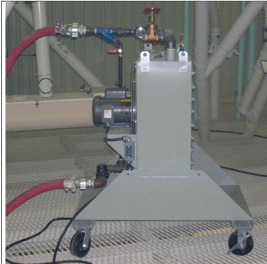
Figure 2. Steam heater (Armstrong International Inc.) used in heat treatment in Mill 3.
